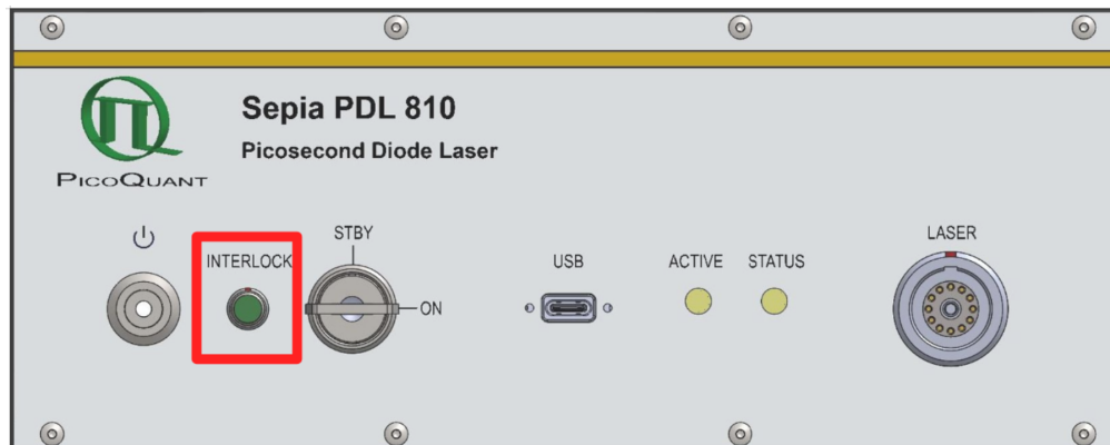
Figure 5: Position of the remote interlock connector on the front panel of the Sepia PDL 810 (highlighted with a red box)
