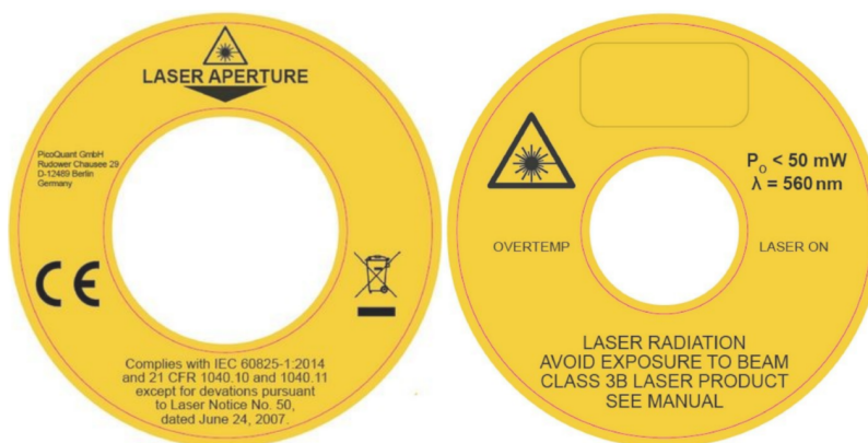
Figure 27: Warning labels for Model type LDH-D-TA-560
