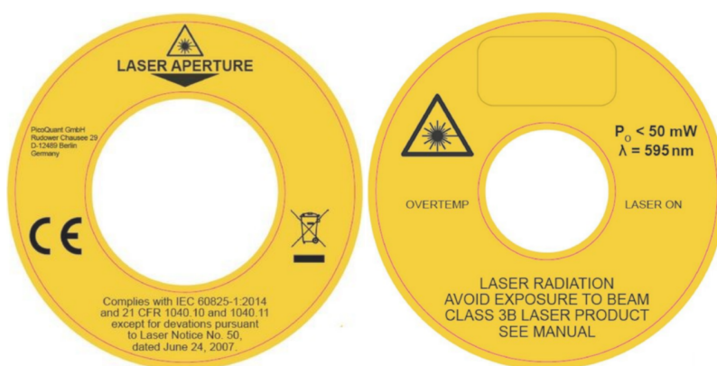
Figure 28: Warning labels for Model type LDH-D-TA-595
