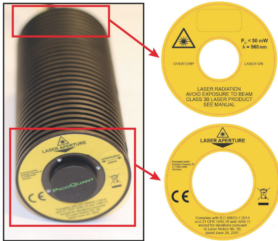
Figure 2: Position of the laser safety, warning labels and aperture indicator on a long cylindrical laser head (LDH-D-TA-530 is used here as an example)
