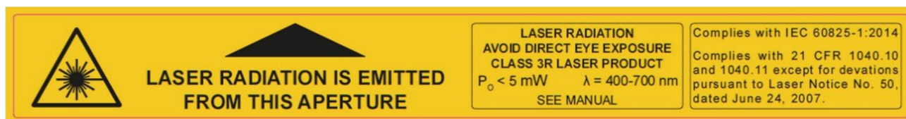
Figure 22: Warning label for LDH lasers with 400-700 nm, P_0 < 5 \text{ mW}
